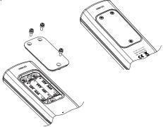
Replace the three 1.5V AAA alkaline batteries located in the battery compartment, observing the indicated polarity.
