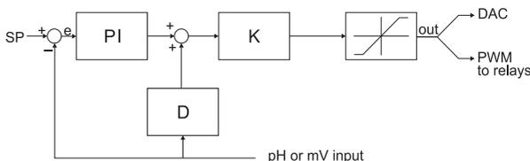
Proportional action can be set by means of the Proportional Band (PB). Proportional Band is expressed in percentage of the input range and is related to  $K_p$  according to the following:
