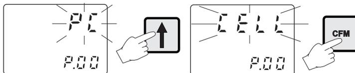
Before enabling this feature it is necessary to enter the PIN of the SIM card of the GSM module (setup item P.01) and one or two phone numbers associated with the service (setup items P.02 and P.03) to which the messages will be sent.
