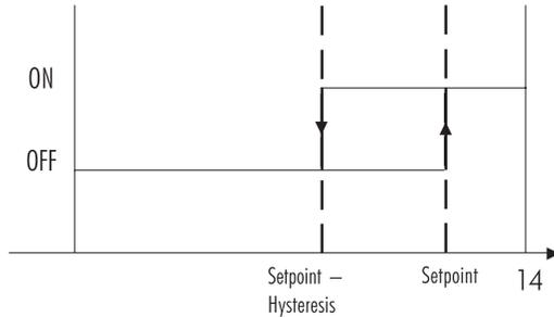
A relay enabled as a low setpoint, is energized when the pH value is below the setpoint and is de-energized when the pH value is above the sum of setpoint and the hysteresis. This operational mode may be used to control an alkaline dosing pump.
