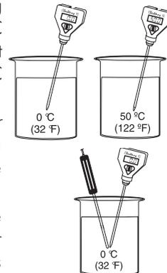
**Note** The instrument can support Pt100 or Pt1000 temperature sensor and calibration can be performed with anyone of these two probes.
