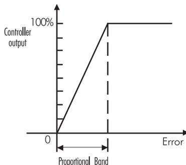
The proportional action is set directly as "Deviation" in pH and mV units respectively. Relation between Deviation (D) and PB is:
