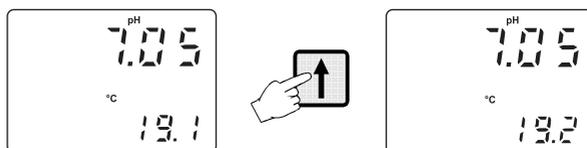
For quickly changing the temperature value press and hold down the  $\hat{\uparrow}$  (or  $\hat{\downarrow}$ ) key: the temperature will be incremented (decremented) of 0.1 °C until the total amount is 0.4 °C, and then the increment (decrement) will turn to 1 °C.
