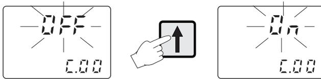
Otherwise, if a numeric value has to be entered for the item, use the  $\uparrow$  or  $\downarrow$  key to change the value of the blinking digit and the  $\rightarrow$  key to cycle through the number's digits.
