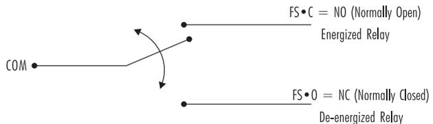
During normal operation (no alarm condition) the alarm relay is energized; during an alarm condition or power failure the relay will be de-energized. As long as a separate battery power system is used an alarm will sound.
