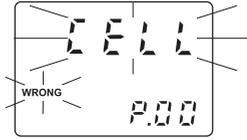
If the PIN set in P.01 is wrong, then it will be not possible to confirm the cellular module connection.
