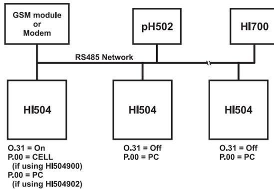
Only one device has to be configured through O.31 to answer to modem calls. That device will be the one controlling the modem or the cellular module. To avoid conflicts, the following must never be done:
