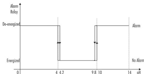
The hysteresis amplitude is 0.2 pH for pH and 30 mV for ORP.
