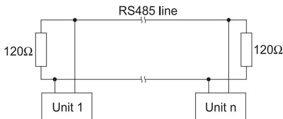
The RS485 can connect up to 31 **HI504** on the same physical network. All the units are slave devices and are monitored and controlled by a single master station (typically an industrial PLC or PC).
