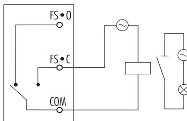
**Note** In order to have the Fail Safe feature activated, an external power supply has to be connected to the alarm device.
