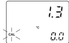
Once confirmed the type of calibration, the primary LCD will display the current temperature measure and the secondary LCD will show the first calibration point (0 °C).
