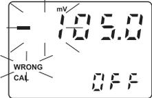
**Note** If LCD or CAL DATA key is pressed before CFM, calibration is aborted without changing the previous calibration data.
