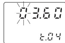
This value is let out to the analog output and coincides with the minimum value of the analog output type chosen with setup item O.11 (analog output 1) and O.21 (analog output 2).
