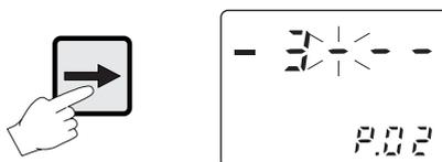
When the fourth digit is reached, by pressing the ⇨ key again, the number on the primary display will scroll of one position to the left and the fifth digit of the phone number will be shown on the fourth position. The minus sign in the front of the number disappears because the shown digits are not the first four ones anymore.
