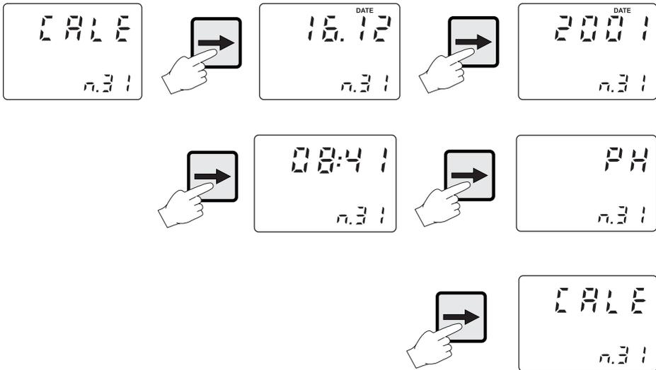
**Note** To exit the log event scrolling, press the LCD key.
