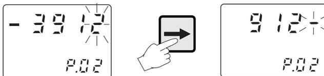
By pressing the ⇧ or ⇩ key it is possible to modify the value of the blinking digit and pressing the ⇨ key it is possible to skip to the next digit. When the end of the phone number is reached, the user has to fill the remaining positions with "-" character.
