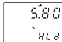
the temperature value can be displayed on the secondary LCD by pressing and holding the ⇨ key; when the ⇨ key is released the “HLd” message comes back on the secondary LCD.
